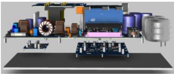
Figure 5: Exploded view of the OBC structure
