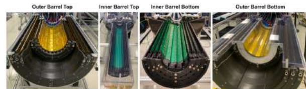
Figure 3: The four Half-Barrels installed in the clean room at CERN during the phase of pre-commissioning [5]
