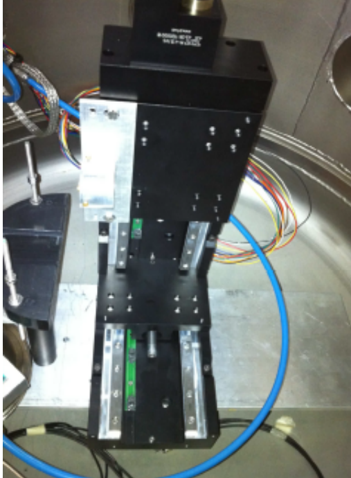
Figure 4: Meccanical scanning for the FARCOS CsI crystals inside the chamber with a collimated ^{241}\text{Am} source.
