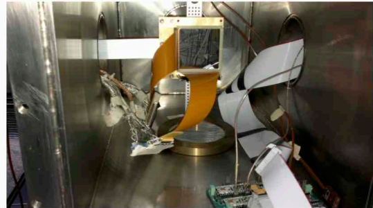
Figure 2: FARCOS DSSSD mounted for test inside of a small chamber at Test-Lab at Sezione di Catania. In the down right corner, it can also be seen a motherboard to manage the signal and supply of two CsI(Tl) crystals.
